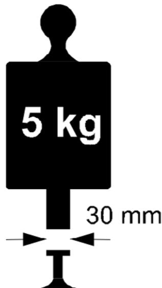
The device used to measure the thickness of clothing and shoes must be capable of measuring to one-tenth of a millimeter (0.1 mm). Measurements must be taken with a 5.0 kg weight applied. The device must have two (2) circular flat surfaces facing each other, each 30 mm in diameter.
